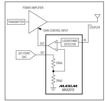
Figure 3. System Diagram for Automatic Gain-Control Loop
