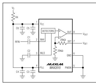
Figure 2. Controller-Mode Typical Application Circuit
