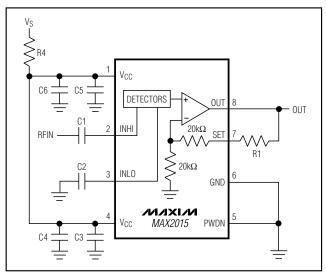
Figure 1. Detector-Mode (RSSI) Typical Application Circuit
